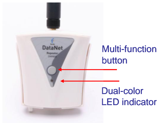
Figure 23: DNR800 Mini Repeater front panel
