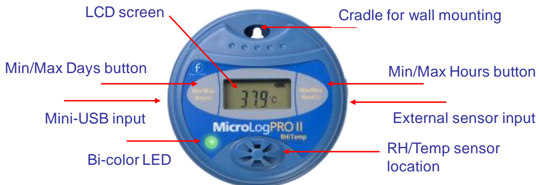
Figure 59: EC850 data logger front panel
